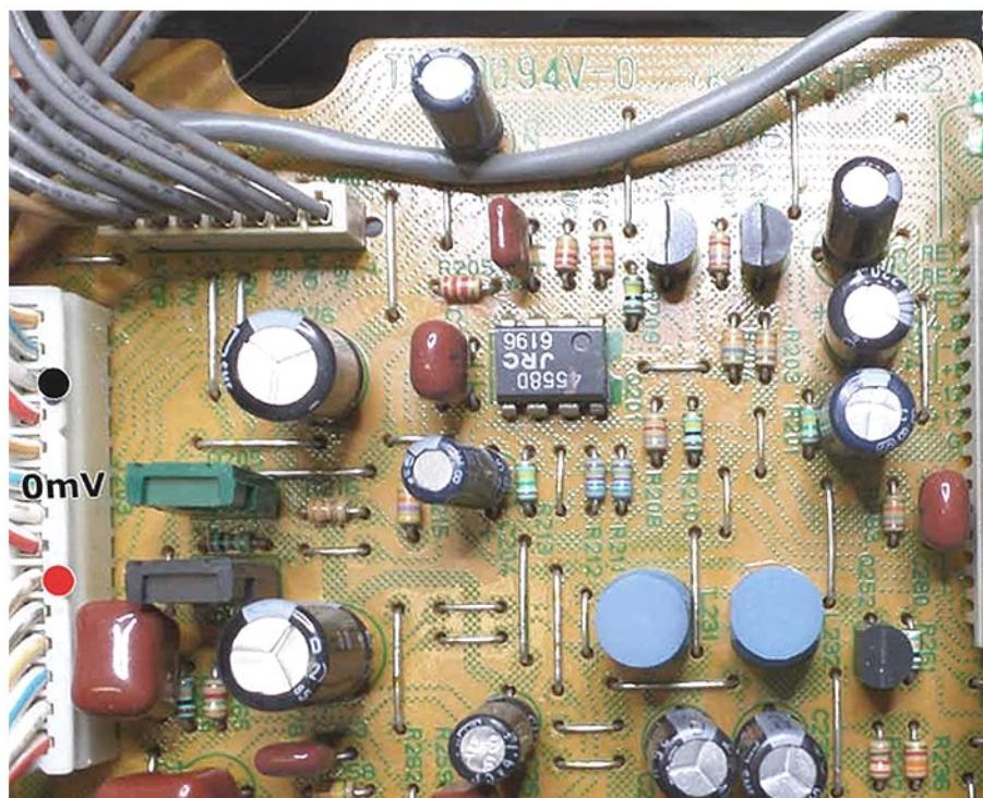
**Measuring points laser voltage: 550 mV**
